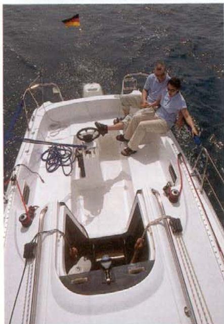
With the small wheel offset to starboard, it can be most comfortable to steer by foot
